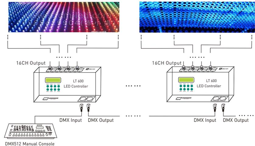
\* DMX console selects the program of controller SD card and controls speed.
