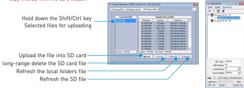
Hold down the Shift/Ctrl key Selected files for uploading
